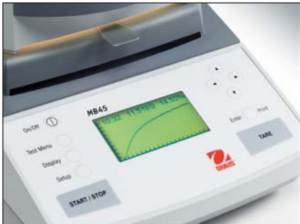
Display shows % moisture, % solids, weight, time, temperature, drying curve and more.
