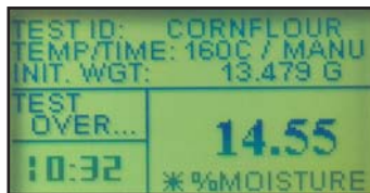
Display shows % moisture, % solids, weight, time, temperature, drying curve and more.
